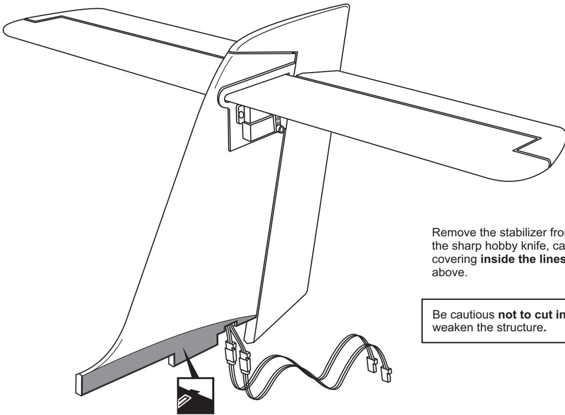
Remove the stabilizer from the fuselage. Using the sharp hobby knife, carefully cut away the covering **inside the lines** which were marked above.
