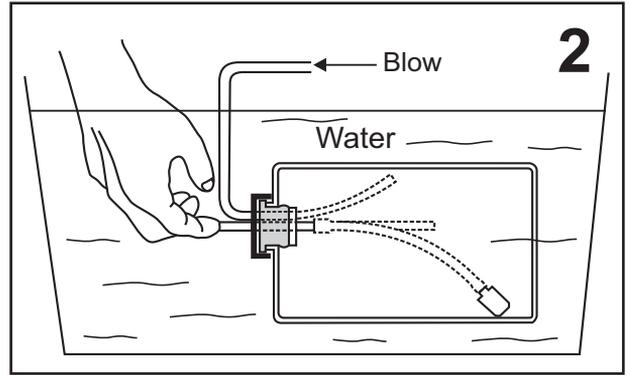
After confirming the direction . Insert this assembly, clunk end first, into the fuel tank and tighten and screw the fuel tank-cap on firmly.
