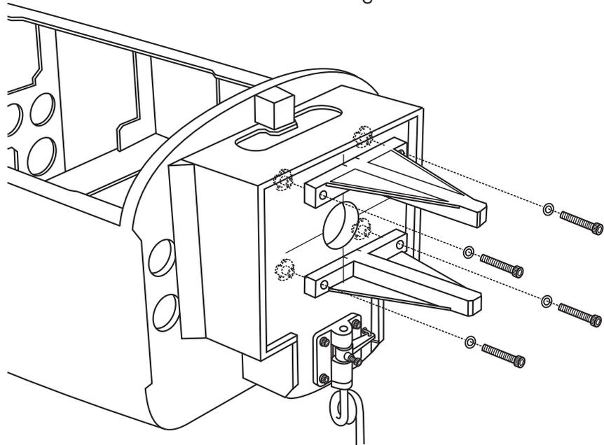
Insert the blind-nut onto each of the four holes make above.
