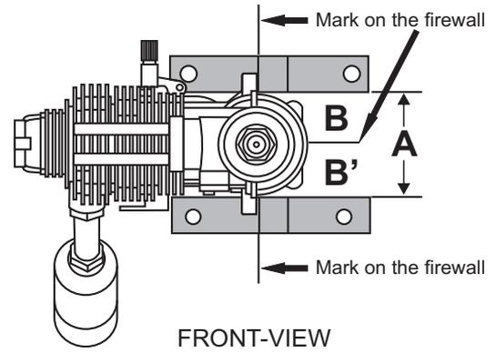
Attach the engine mount beams onto the fire-wall so the distance between of two engine mount beams is "A", and B=B' as show. Secure the engine mount beams onto the fire-wall with litter CA glue
