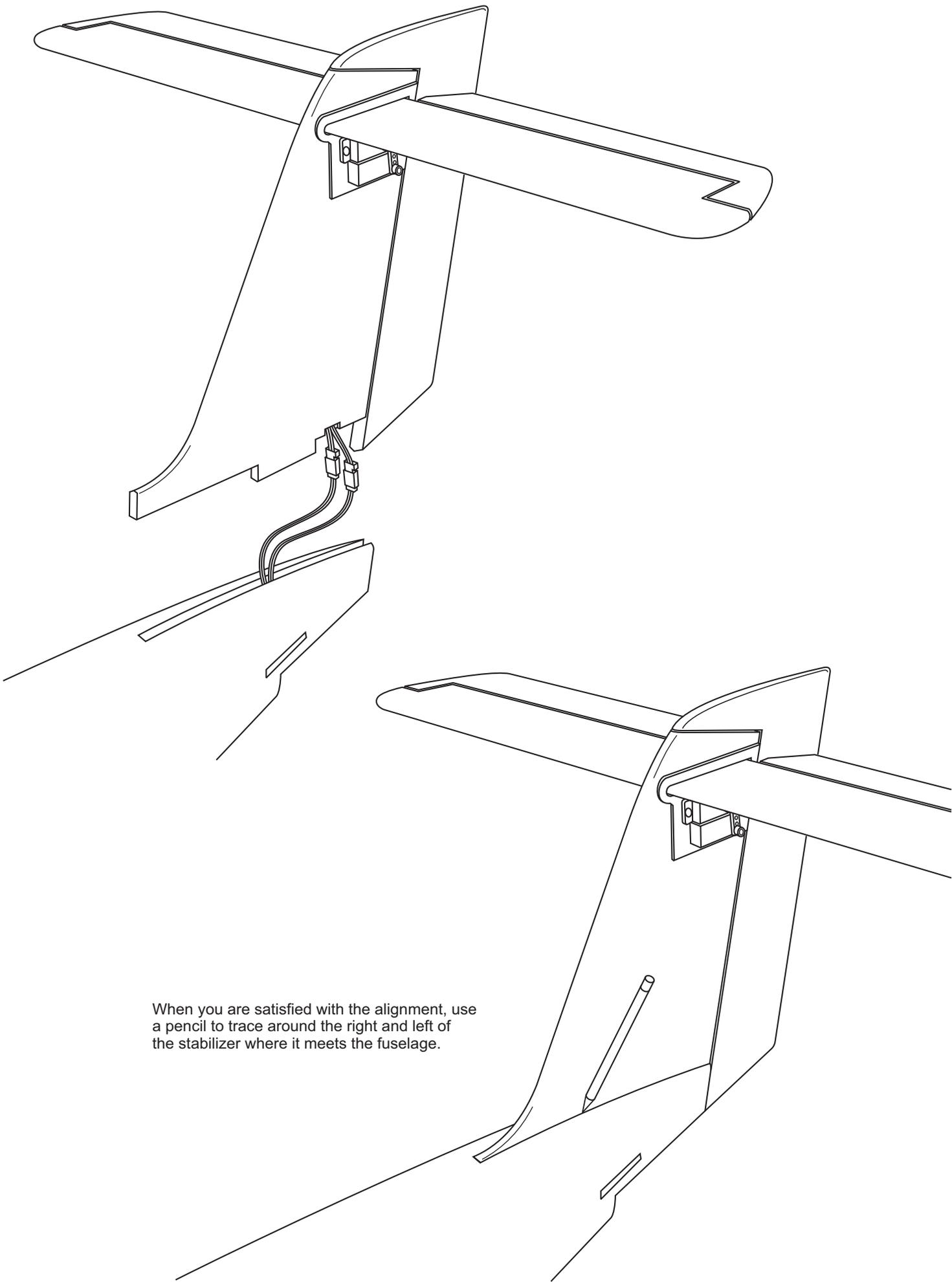
When you are satisfied with the alignment, use a pencil to trace around the right and left of the stabilizer where it meets the fuselage.
