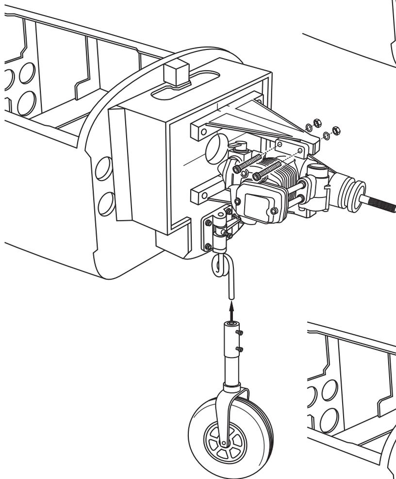
Reposition the engine on the engine mount beams, aligning it with the holes. Secure the engine to the engine mount using four 3x25mm hex bolts.
