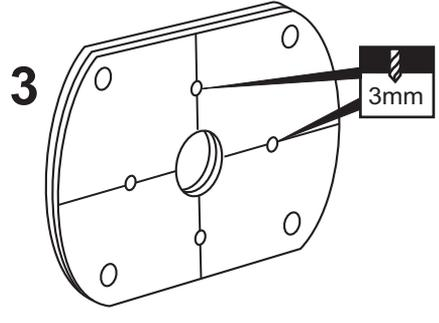
Using a aluminum motor mounting plate as a template, mark the plywood motor mounting plate where the four holes are to be drilled.
