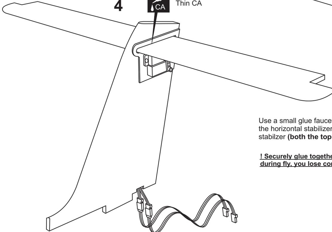
Use a small glue faucet, Apply the thin CA glue on the horizontal stabilizer where it contacts the vertical stabilizer (**both the top and bottom sides**).
