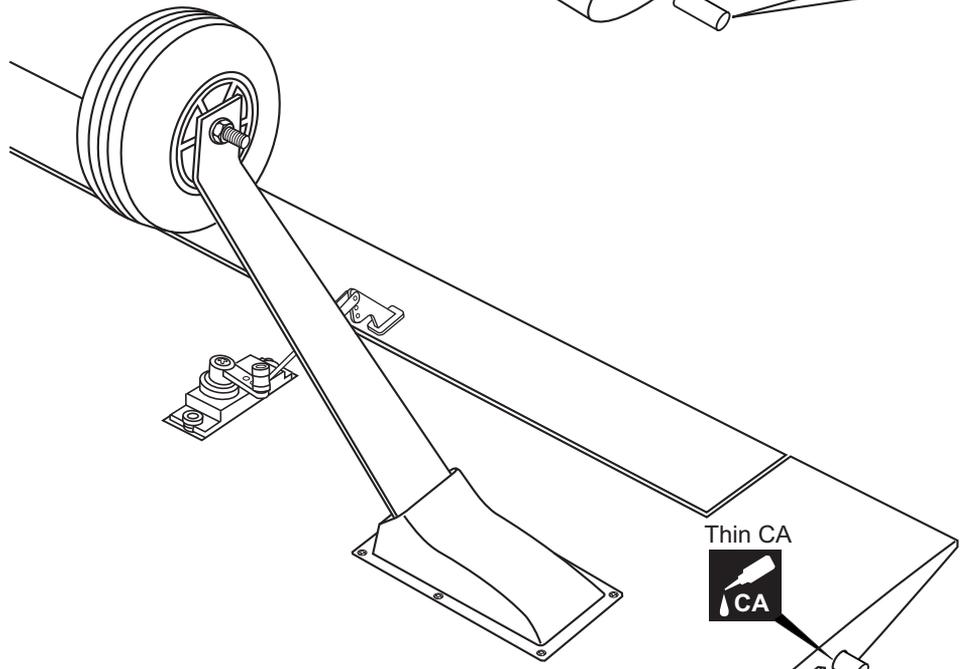
**Note:** Make sure that the dowel must be perpendicular with the wing root before glue.
