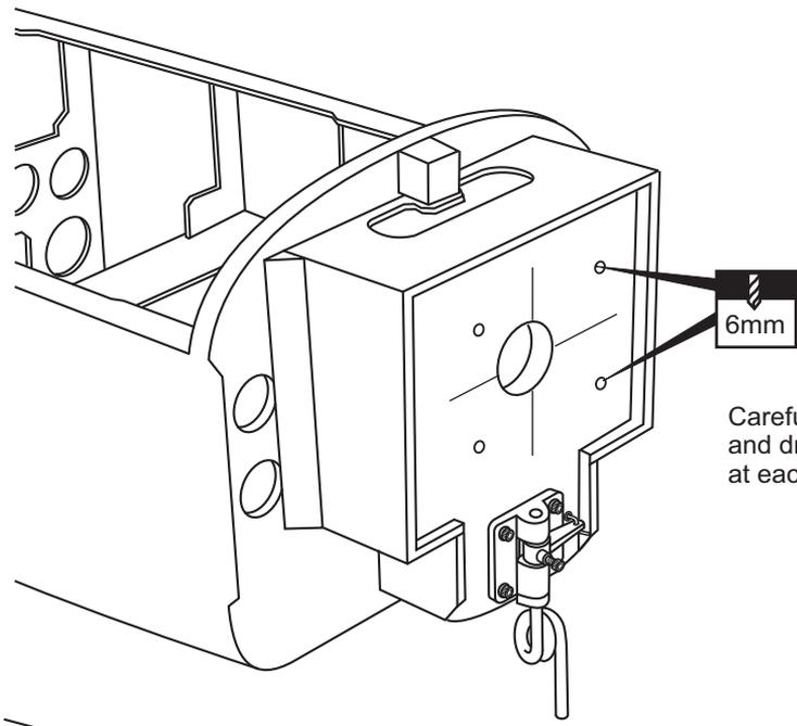
Carefully remove the engine mount beams and drill a 6mm hole through the fire-wall at each of the four marks made above.
