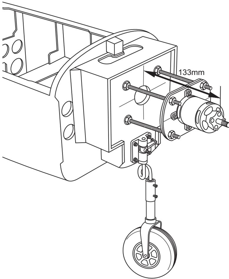
Position the motor mount to so the distance from the prop hub to the fire-wall is 133mm .
